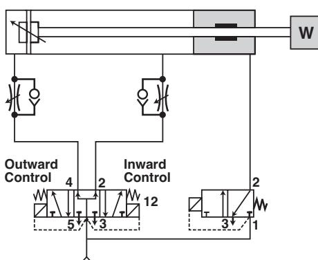
System shown: vertical mounting with the load beneath the cylinder
