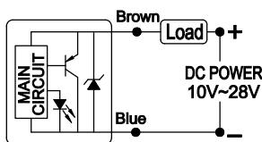
The brown wire series load to the positive (+) and the blue to the negative (-) of power source.
