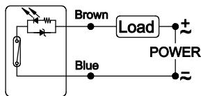
The brown wire series load to the positive (+) and the blue to the negative (-) of power source.
